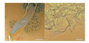
Left: TEM cross section of Mn oxide on a hypha of the fungus, Plectosphaerella cucumerina. Right: HR-TEM image showing Mn oxide with a rumpled, sheet-like morphology.
