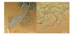
Left: TEM cross section of Mn oxide on a hypha of the fungus, Plectosphaerella cucumerina. Right: HR-TEM image showing Mn oxide with a rumpled, sheet-like morphology.
