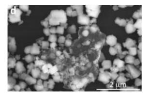
High resolution SEM image after colloidal processing indicating partially exfoliated GPL mixed with well-dispersed Si3N4 particles. The images clearly indicate GPL decorated with Si3N4 particles; the Si3Nk4 particles are welldispersed throughout the surface area of the sheets. Credit: ACS Publications/UA Engineering
