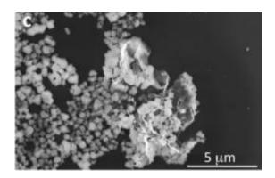
This is a low resolution SEM image after colloidal processing indicating partially exfoliated GPL mixed with well-dispersed Si3N4 particles. The images clearly indicate GPL decorated with Si3N4 particles; the Si3Nk4 particles are well-dispersed throughout the surface area of the sheets. Credit: ACS Publications/UA Engineering
