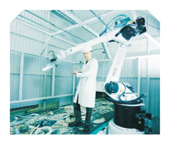
(PhysOrg.com) -- The Finnish firm ZenRobotics has designed and built a robot that can sort through construction waste and pluck out recyclable material moving by on conveyer belt and then deposit it in an appropriate bin. The robot is currently able to correctly identify roughly
