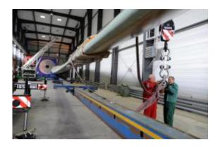
The new facility will enable the institute's engineers to perform load tests on rotor blades measuring up to 90 meters in length.
