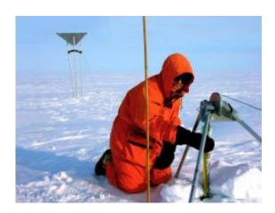
Taking in situ measurements of ice and snow are an essential part of the calibration and validation programme for the CryoSat mission. Here a neutron probe is lowered into a hole drilled in the ice. It collects essential data on snow and ice density layering to help understand the radar signals from the satellite and ultimately transform the height measurements into net change in ice mass, the main goal of CryoSat. Credits: Norwegian Polar Institute
