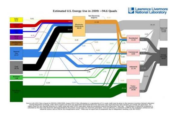
This flow chart shows the amount of energy (in quads) that is produced by different energy sources and consumed by different sectors. Image credit: Lawrence Livermore National Laboratory and the US Department of Energy.
