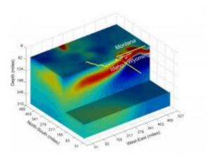
This image, based on variations in electrical conductivity of underground rock, shows the volcanic plume of partly molten rock that feeds the Yellowstone supervolcano. Yellow and red indicate higher conductivity, green and blue indicate lower conductivity. Made by University of Utah geophysicists and computer scientists, this is the first large-scale "geoelectric" image of the Yellowstone hotspot. Credit: University of Utah.
