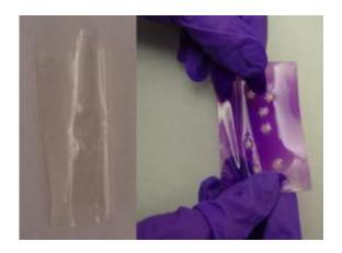
The image to the left shows one of the photochromic gels before exposure to UV light. The image on the right shows the elastic material after exposure to UV light. Credit: Jan Genzer, North Carolina State University
