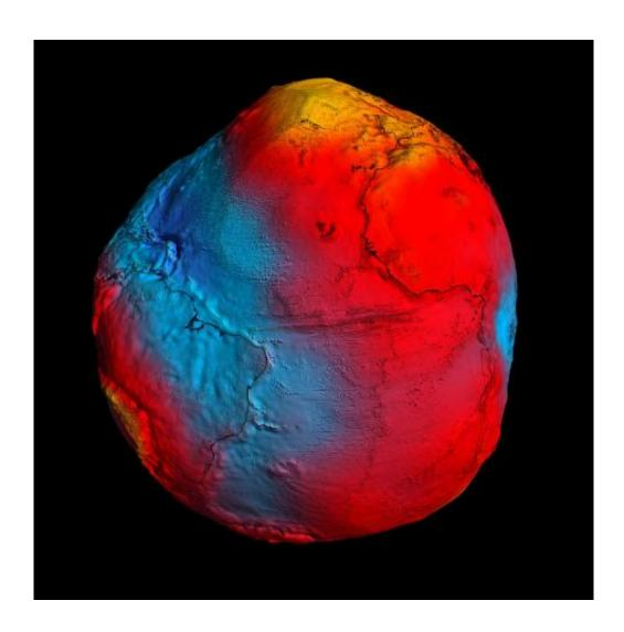
ESA's GOCE mission has delivered the most accurate model of the 'geoid' ever produced, which will be used to further our understanding of how Earth works. A precise model of Earth's geoid is crucial for deriving accurate measurements of ocean circulation, sea-level change and terrestrial ice dynamics. The geoid is also used as a reference surface from which to map the topographical features on
