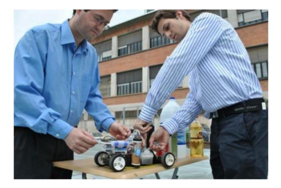
(PhysOrg.com) -- Aleix Lovet and Xavier Saluena, two researchers at the Polytechnic Institute of Catalonia, have made the world first RC car that runs entirely on soda cans. Well, to be more accurate, it runs on a combination of recycled aluminum soda can tabs and sodium hydroxide. This creates a vehicle that is completely carbon emission free and creates no planet harming waste.
