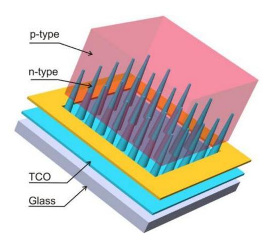
Nanocone-based solar cell consisting of n-type nanocones, p-type matrix, transparent conductive oxide (TCO) and glass substrate.
