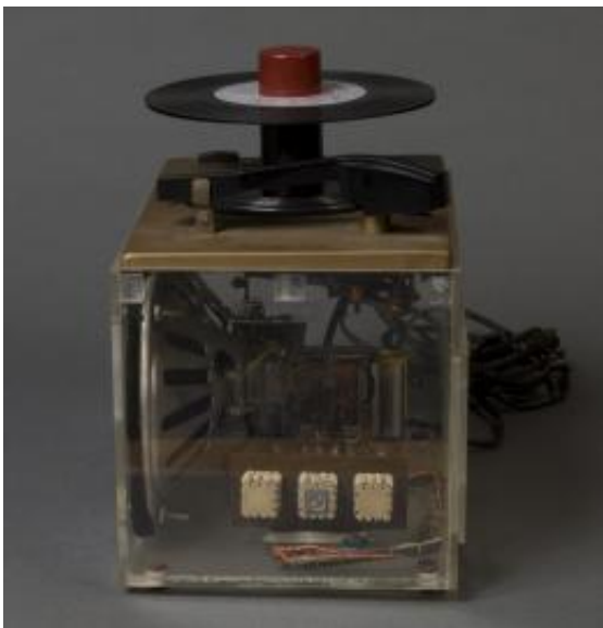
Project Tinkertoy Wafer Tube Amplifier. Credit: NIST Digital Archives
