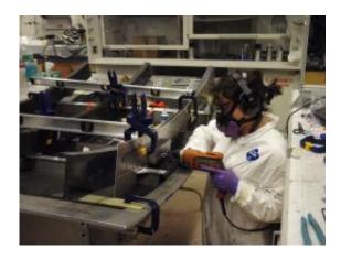
UC San Diego structural engineering grad student Gabriela DeFrancisci has been testing damage to composite aircraft materials from hail, ice and ground service equipment vehicles.
