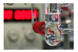
Using a molybdenum based catalyst, hydrogen bubbles are made cheaply and at room temperature. Credit: EPFL / Alain Herzog
