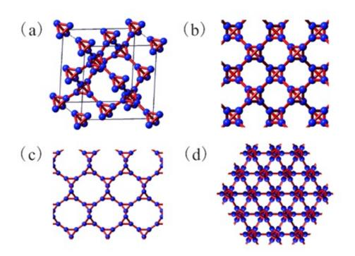
The structure of the new carbon allotrope, T-carbon, is shown from different directions. T-carbon is obtained by replacing each carbon atom in diamond with a carbon tetrahedron. Image credit: Sheng, et al. ©2011 American Physical Society.
