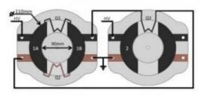
This is a schematic of the physical layout of the soft generator. Credit: N/A
