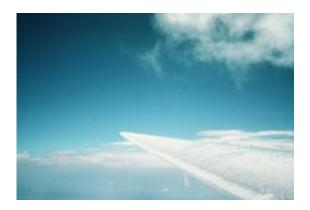
This image shows icing buildup on the wing of a small aircraft. Credit: ©UCAR. This image is freely available for media use.
