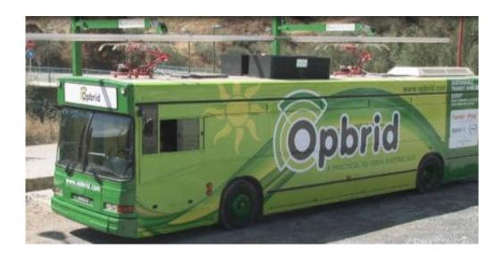
(PhysOrg.com) -- The Spanish "green" technology firm, Opbrid, has delivered a new kind of diesel-electric hybrid commuter bus to the northern Swedish town of Umea for initial testing of its over-head fast charging vehicle, dubbed the "Arctic Whisper." The name comes from the fact that it is almost silent as it makes its way around and the fact that onboard it's so quiet, you can actually whisper to a fellow traveler.
