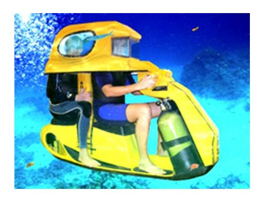
The AS-2 Scooter can seat two people at a time, which is an improvement over the previous model. It features an improved helmet which allows the user to have a 99% distortion free view of the ocean. This model is also both lighter and faster than its predecessor, which allows users to go farther in the same span of time, and between the air
