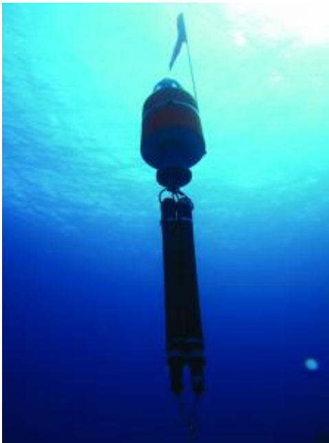
An ecological acoustic recorder (EAR) used to record humpback whale song. Credit: NOAA PIFSC
