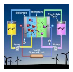
This artist's rendering of an upgraded vanadium redox battery shows how using both hydrochloric and sulfuric acids in the electrolyte significantly improves the battery's performance and could also improve the electric grid's reliability and help connect more wind turbines and solar panels to the grid. Credit: Pacific Northwest National Laboratory
