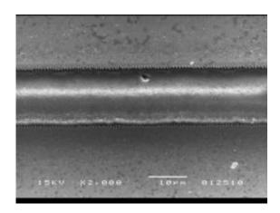
This image, taken with a scanning electron microscope, shows a microchannel that was created using an ultrafast-pulsing laser. Credit: Purdue University School of Mechanical Engineering image/Yung Shin
