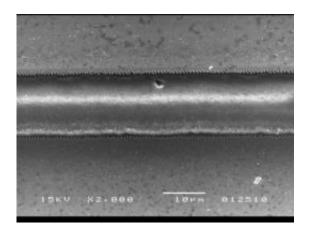
This image, taken with a scanning electron microscope, shows a microchannel that was created using an ultrafast-pulsing laser. Credit: Purdue University School of Mechanical Engineering image/Yung Shin
