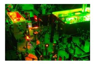
Laser system for generating ultra short x-ray pulses which is used in the experiment to make the recordings. Photo: Rohwer et al., Copyright: CAU
