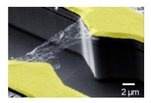
Single-walled carbon nanotubes are promising building blocks for future optoelectronic devices. With this measurement set-up physicists led by Professor Alexander Holleitner (Technische Universitaet Muenchen) can resolve the ultra fast optoelectronic dynamics of carbon-nanotubes. A first laser exites electrons in the carbon-nanotubes spanning the gap between two gold electrodes while a second laser measures the resulting photo-current. Credit: Prof. Dr. A. Holleitner, TUM
