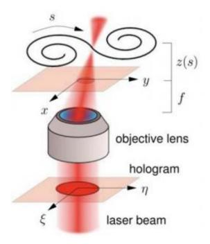
A laser beam is imprinted with a hologram in the input pupil of an objective lens. The hologram is projected through the objective's focal plane and comes to a focus along a 3-D curve parameterized by its arc length, s. Credit: Optics Express
