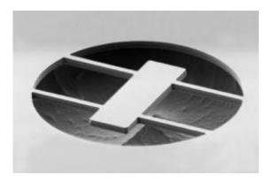
Researchers at the University of Vienna and the Technische Universitaet Muenchen have solved a long-standing problem in the design of mechanical resonators: the numerical prediction of the design-limited damping. The electron microscopic picture shows one of their micro resonators with which they proved the performance of their calculations. Credit: Garrett Cole, University Vienna
