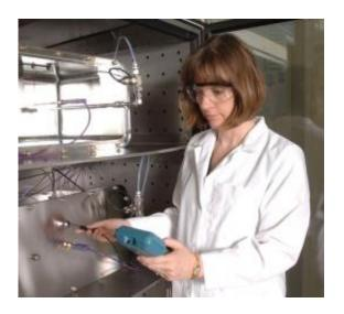
At NIST's small chamber test facility, researchers are assessing the performance of a prototype reference material for testing emissions of VOCs from building products. Credit: NIST
