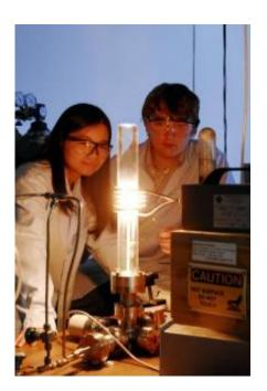
Georgia Tech graduate students Yike Hu and John Hankinson observe a hightemperature furnace used to produce epitaxial graphene on a silicon carbide wafer. A new "templated growth" technique allows fabrication of nanoribbons with smooth edges and high conductivity. Credit: Georgia Tech Photo: Gary Meek
