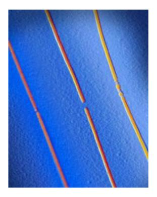
Three parallel memory bits with carbon nanotube electrodes (false color image based on topographic profile from atomic force microscopy). The middle bit is in the "off" state, the other two are "on". The silicon dioxide substrate is shown in blue. Credit: Eric Pop, University of Illinois
