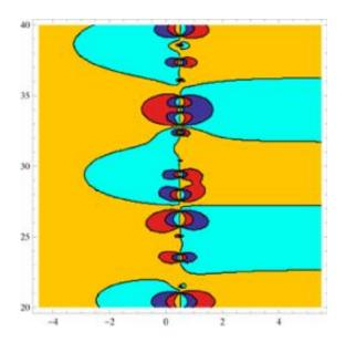
Different colours in this image mark regions of different phase of an angular lattice sum divided by the basic two-dimensional sum. The light blue areas must contain exactly the same numbers of zeros of each function, proving important properties of each.
