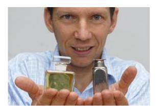
Jan Schroers and his team have developed novel metal alloys that can be blow molded into virtually any shape.
