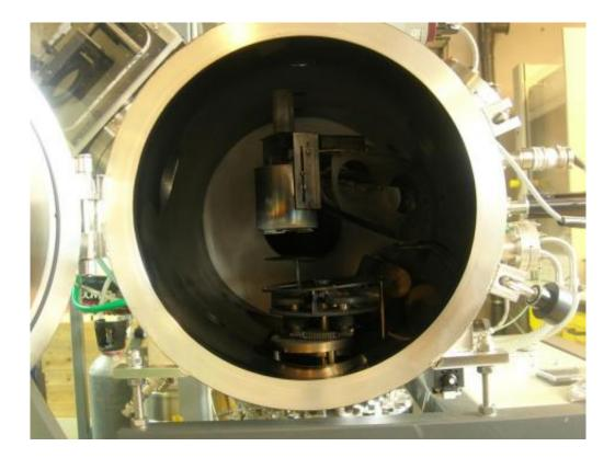
This chamber is used by scientists at the Max Planck Institute for Microstructure Physics to produce the ferroelectric material PZT using pulsed laser deposition (PLD). The method permits extremely accurate control of the material formation. © MPI of Microstructure Physics
