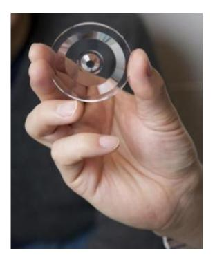
A lens invented at Ohio State University enables microscopes to capture 3-D images of tiny objects. Credit: Photo by Kevin Fitzsimons, courtesy of Ohio State University.
