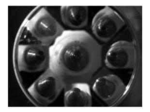
Researchers at Ohio State University have invented a 3-D microscope lens that gathers images of tiny objects from nine different angles at once. Here the lens captures a ballpoint pen tip that measures about 1 millimeter across. Credit: Image courtesy of Ohio State University.
