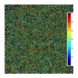
This is an orientation map of a spin-cast array of FePt nanoparticles. Most nanoparticles are enclosed by a hexagon of six neighboring nanoparticles. Each nanoparticle was color coded according to the angle (in degrees) of the hexagon's orientation. Nanoparticles colored white were identified as defects, because they had four, five, seven or eight "nearest neighbors" -- rather than six. Credit: Dr. Joe Tracy, North Carolina State University
