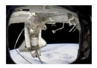
In this image provided by NASA the docked space shuttle Discovery and the Canadian-built Special Purpose Dextrous Manipulator, are photographed by a crew member on the International Space Station. The blackness of space and Earth's horizon provide the backdrop for the scene. This is the last time the Shuttle Discovery will dock with the International Space Station. (AP Photo/NASA)
