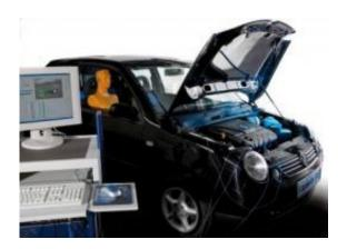
Researchers are testing oscillation-damping piezo bearings aboard a VW Passat. Credit: Fraunhofer LBF
