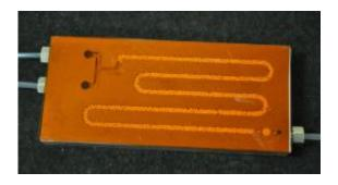
Typical NIST microreactor plate for studying enzyme catalyzed polymerization. The aluminum plate, topped with a transparent film, is approximately 40 mm by 90 mm centimeters. The channel, filled with plastic beads carrying the enzyme catalyst, is 2 millimeters wide and 1 deep. Credit: Kundu, NIST
