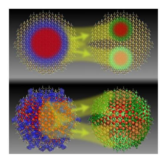
Illustration of multiple-exciton generation (MEG), a theory that suggests it is possible for an electron that has absorbed light energy, called an exciton, to transfer that energy to more than one electron, resulting in more electricity from the same amount of absorbed light. The left side shows an electron promoted to a high energy state (blue) plus the "hole" vacated by the electron (red). The right side shows the original exciton (now dark green/red) and a new exciton (light
