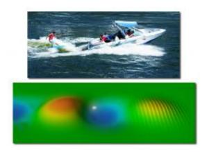
Like a speedboat leaving a wake that a surfer can ride, a laser pulse in a laser-plasma wakefield accelerator creates a wake in the plasma that an electron beam "surfs" to high energy. The ridges at bottom right are the laser pulse, which drives the wake as it speeds through the plasma. Colors in the wake represent intense electric fields: the decelerating fields (orange) and accelerating fields (blue) drive the electrons (white) to high energy. (Original boat-surfing photo by Sean C. Fulton)
