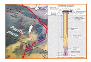
Left: An aerial view of the area where seismic images are being collected. Heavy red lines indicate the San Andreas and related faults. Seismic charges will be detonated at the bottom of a cased drill hole, illustrated at right. Credit: USGS
