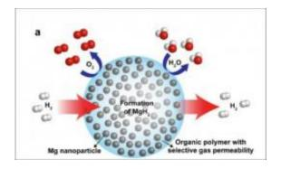
This schematic shows high-capacity magnesium nanocrystals encapsulated in a gas-barrier polymer matrix to create a new and revolutionary hydrogen storage composite material. Credit: Image from Jeff Urban
