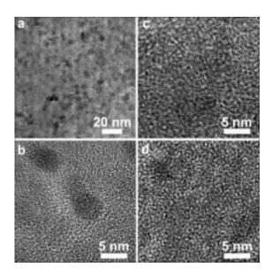
Transmission electron micrographs of an air-stable composite comprised of metallic magnesium nanocrystals in a gas-barrier polymer matrix that enables the high density storage and rapid release of hydrogen without the need for heavy, expensive metal catalysts. Credit: Images from National Center for Electron Microscopy
