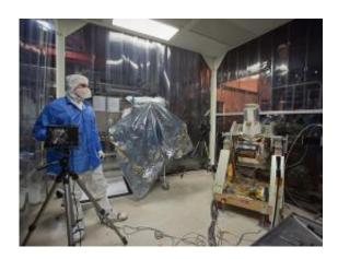
NASA Langley engineer Mark Thornblom helps calibrate SAGE III-ISS for its scan of the moon Feb. 17. The SAGE team arrived at midnight to continue testing the instrument, which will be attached to the space station to measure ozone, water vapor and aerosols in the Earth's atmosphere. Credit: NASA/Sean Smith
