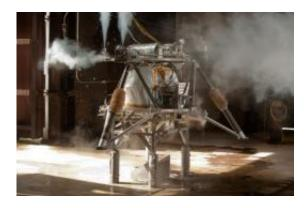
The robotic lander during strapdown testing. This phase of tests allows the engineering team to fully check out the integrated lander prototype before moving to more complex free flight tests. Credit: NASA/David Higginbotham
