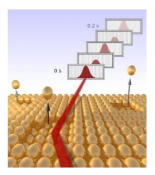
Graphical representation of the experiment. The X-ray beam impinges on a gold surface, which is chemically dissolving. A fast X-ray detector captures the reflected beam. From the fluctuations of the beam intensity with time, the atomic-scale changes at the surface are deduced. Copyright: CAU, artwork: J. Golks
