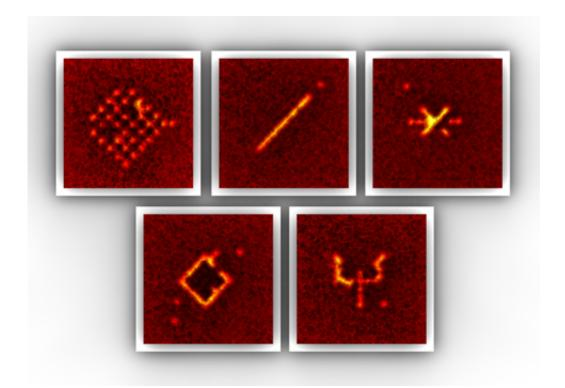
With the addressing scheme arbitrary patterns of atoms in the lattice can be prepared. The atomic patterns each consist of 10 - 30 single atoms that are kept in an artificial crystal of light.
