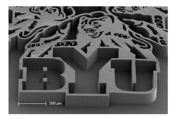
BYU physicists made this tiny logo as a demonstration of their technique for growing stable structures from carbon nanotubes.
