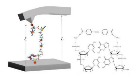
(Left) An illustration of the DNA-based molecular motor. The molecule is extended in its soft cis mode, and then contracted back to its original size in its stiffer trans mode, when work is extracted. (Right) An illustration of the DNA's structure. Image credit: McCullagh, et al. ©2011 American Chemical Society.
