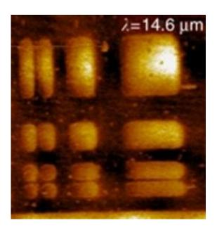
This atomic-force microscopy image shows the strontium ruthenate rectangles that were imaged with perovskite-based superlens using incident IR light of 14.6 micrometer wavelengths. Credit: Image from Kehr, et. al
