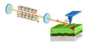
Experimental setup shows an IR free-electron laser light source and perovskite superlens consisting of bismuth ferrite (BiFeO3) and strontium titanate (SrTiO3) layers. Imaged objects are strontium ruthenate patterns (orange) on a SrTiO3 substrate. The near-field probe is shown in blue and the evanescent waves in red. Credit: Image from Kehr, et. al
