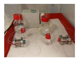
The experimental set-up shows two diffusion cells with built-in clay cylinders and vials with pore water containing neptunium and plutonium respectively. In the background there is a peristaltic pump. Credit: Institute of Nuclear Chemistry
