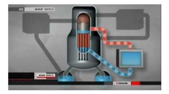
This illustration of a nuclear reactor shows water entering the core and surrounding the fuel rods (vertical red bars). When the water level decreases, the fuel rods begin to heat up and face the risk of melting. Image from video below.
